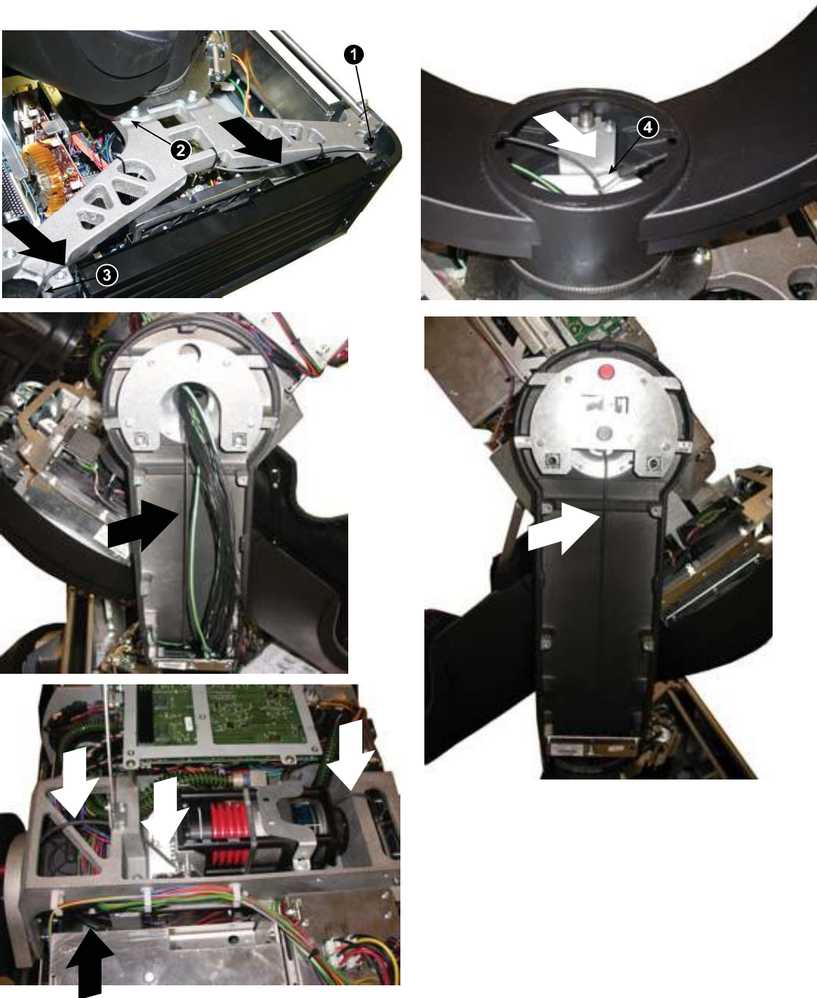
Image 13-5 Internal safety cable, routing
